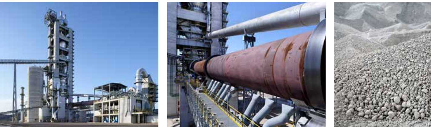
Cement plant with co-processing functionality (left), rotary cement kiln (centre) and output clinker (right).
